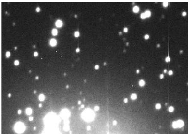
Figure 75. Example subsection of a science image. The target is the hPersei open cluster and problematic CCD columns are noticeable as vertical smears affecting some stars.
