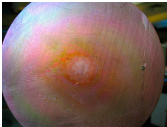
Collector plate erosion
